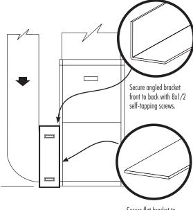
Secure flat bracket to bottom or back with 8x1/2 self-tapping screws.
